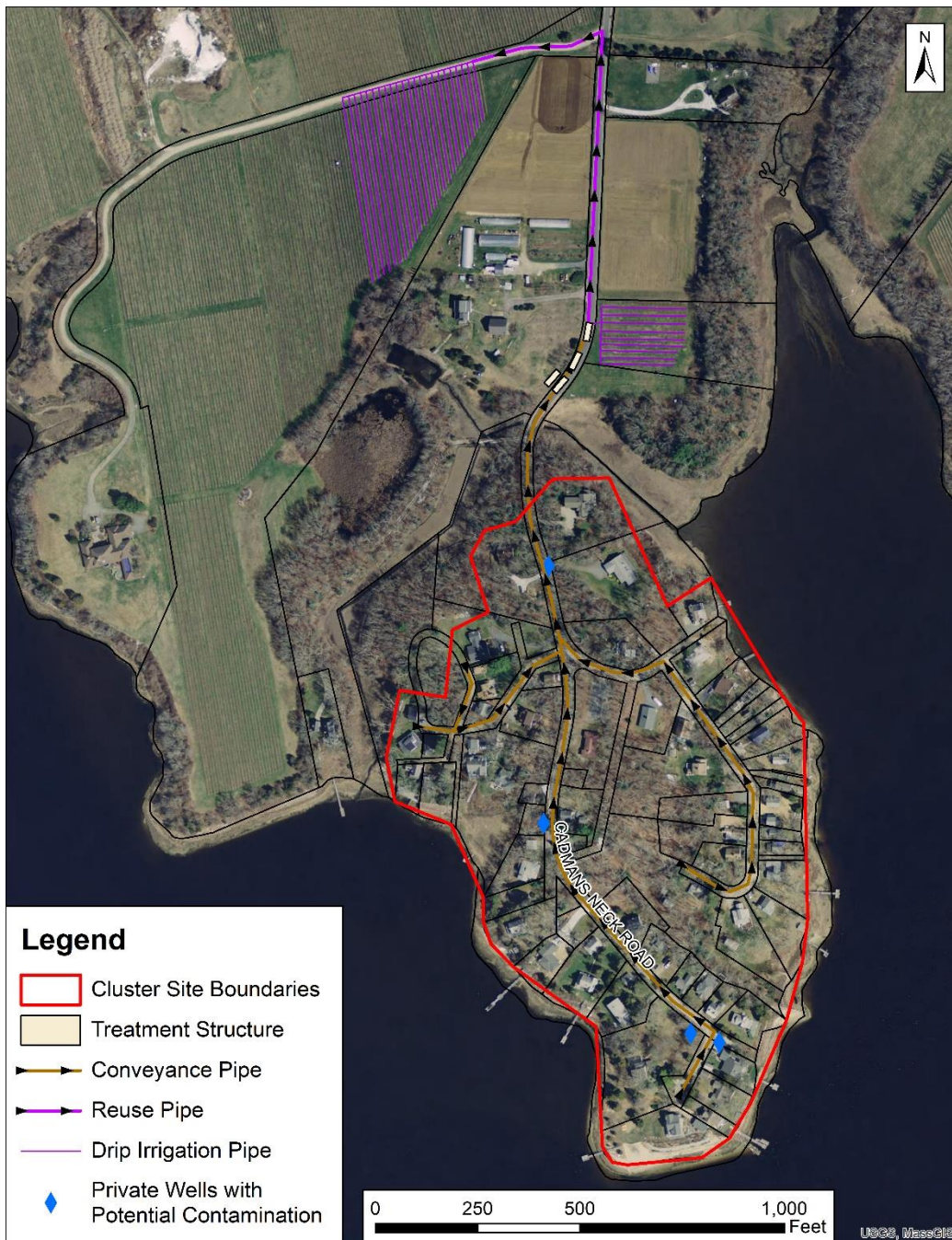
Figure 8.4. Conceptual Design for Cluster Septic Systems at Cadman’s Neck
