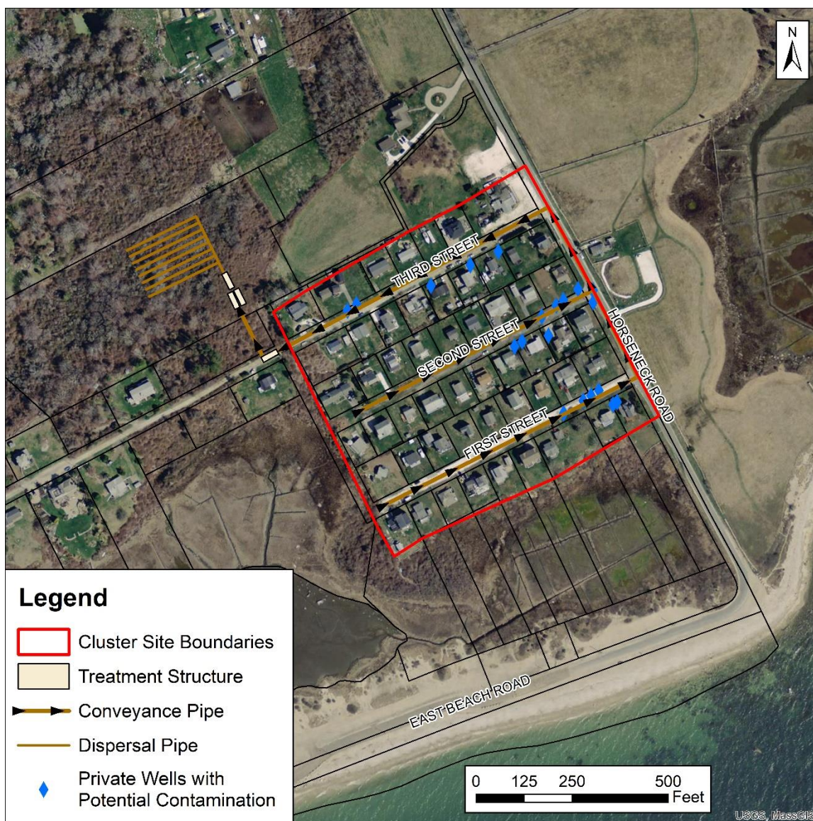
Figure 8.5. Conceptual Design for Cluster Septic Systems at The Let
